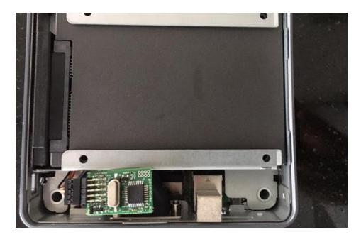
• After attaching the wiring loom, you can store the connected PCB as shown
