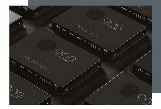
The OneIP family is the result of four years of relentless innovation and development, a full duplex Video over IP transceiver at 1Gbps.
